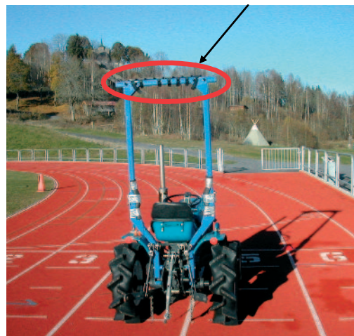
Figure 1. The running track, the minitractor and the GPS units mounted on the traverse.
