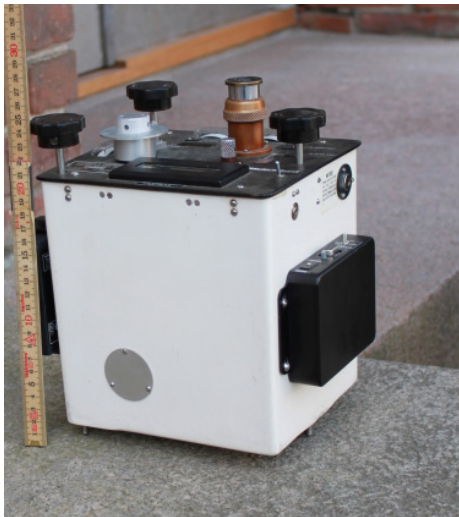
Figure 3: LCR G-761 set up on the stone stairways at CI01.
