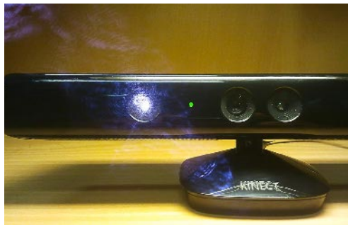
Figure 2: Taking a picture with a mobile phone of the front of the kinect while it is recording reveals the IR-beamer. The middle lens is the RGB-camera, and the one on the right is the IR-camera.
