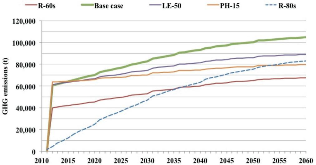
Figure 1 GHG emissions of various new construction and renovation options during a 50-year time frame (Säynäjoki A. et al. 2012)
